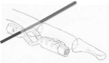
Figure: Bracket is slid over the axis pin.
