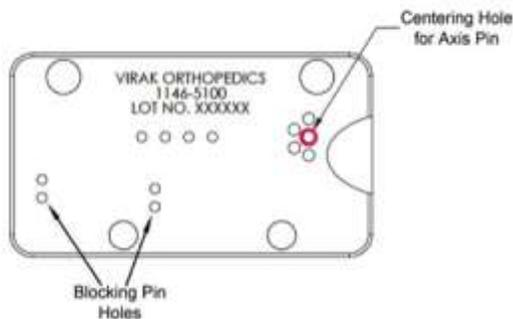
Figure: Diagram of the pin guide showing the Centering Hole and Block Pin Holes.
