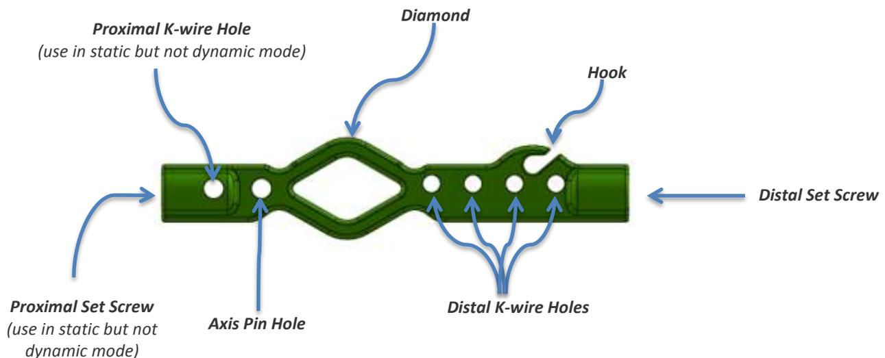
Figure: Diagram of the DigiFix® Bracket.
